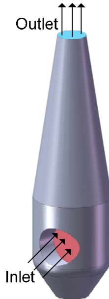
Figure 3 – SFM Internal Geometry
